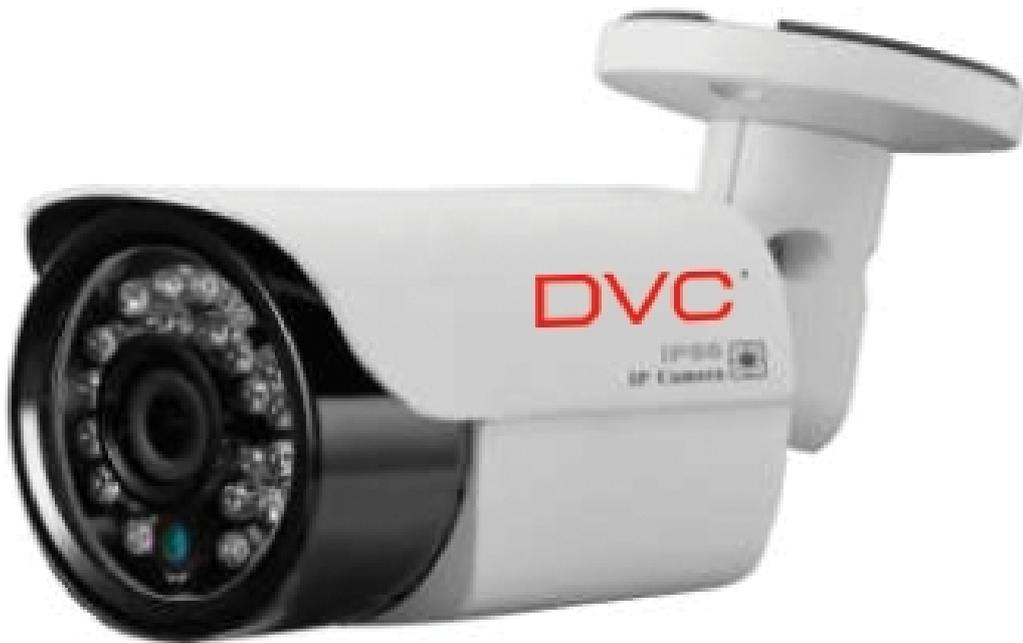
**AHD 2.0 vanjska kompaktna dan/noć IR kamera, 1/2.8" Sony EXMOR CMOS, rezolucija 1080p, objektiv 2.8 mm, D-WDR, osjetljivost 0 Lux IR ON (0.017Lux IR OFF), 48 IR Led dometa 20-30 m, napajanje 12VDC, IP65.**
