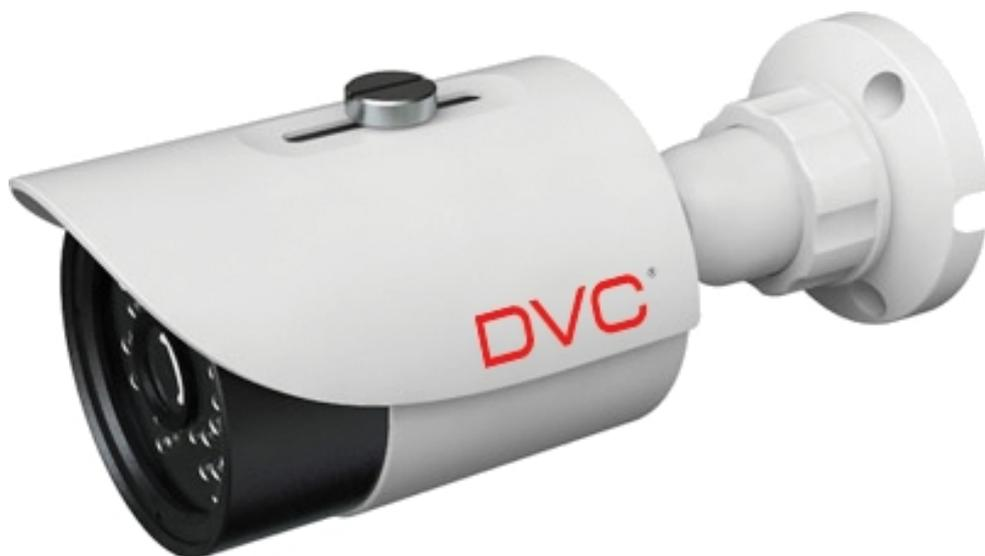
**Vanjska kompaktna IP video kamera, 2Mpx/25fps, 2.8 - 12 mm, H.264, ICR, IC LED 20-30 m, 12VDC/PoE, audio in, Onvif.**
